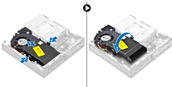
4. Disconnect the speaker cable and system fan cable from the connectors on the system board.
