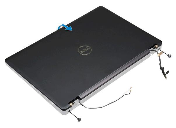
**c.** Lift the display assembly from the computer.
