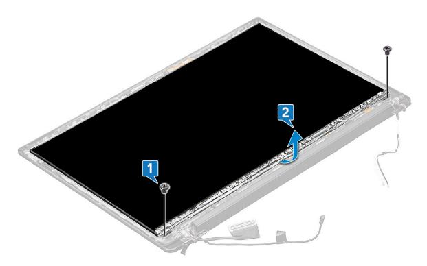
c. Slide the display panel away from the system from the bottom [1], and flip the display panel over [2].
